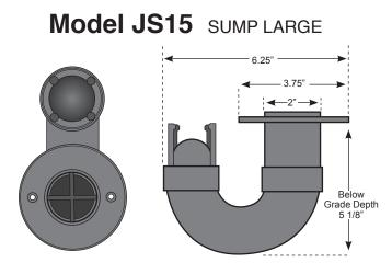
Fits into and becomes part of your sump cover. It is a one way valve that allows water to flow into the sump but prevents Radon Gas, soil gas, insects and odours from entering your living environment.
