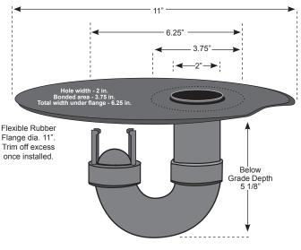
For large floor drains. The unit fits underneath the existing strainer plate and is held in place by friction (pinched between the strainer plate and the retaining ring) and by caulking.
